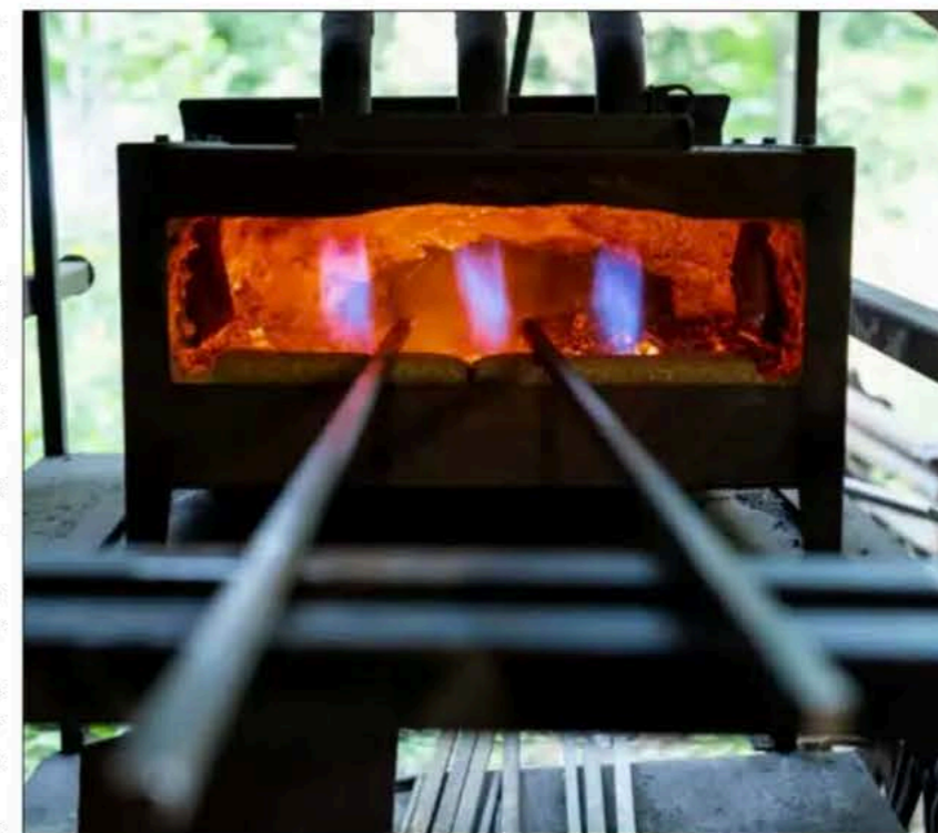
Top: The colour of iron is important in a blacksmith's shaping process. A bright yellow-orange is the best for forging and welding. Above: When the shop originally opened, The Smithy used a coal forge to heat metals, sometimes taking all day to reach the appropriate temperature. Now, it's gas-fired.
